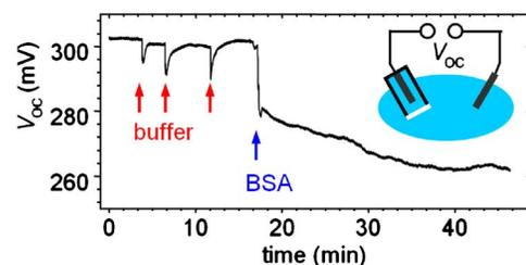
FIG. 3. (Color online) Open-circuit voltage of a Ag/AgCl reference electrode in series with a bare Pt wire. The buffer solution and BSA protein solution are the same as used in Fig. 1.
