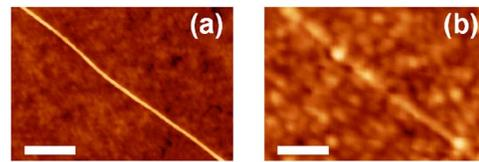
FIG. 2. (Color online) Nonspecific adsorption of BSA protein on a CNT and silicon oxide surface. (a) Before exposure to protein. (b) After 60 min incubation in protein solution ( $10 \mu\text{M}$  BSA in phosphate-buffered saline). In both images, the height scale is 3.5 nm and scale bars are 100 nm.
