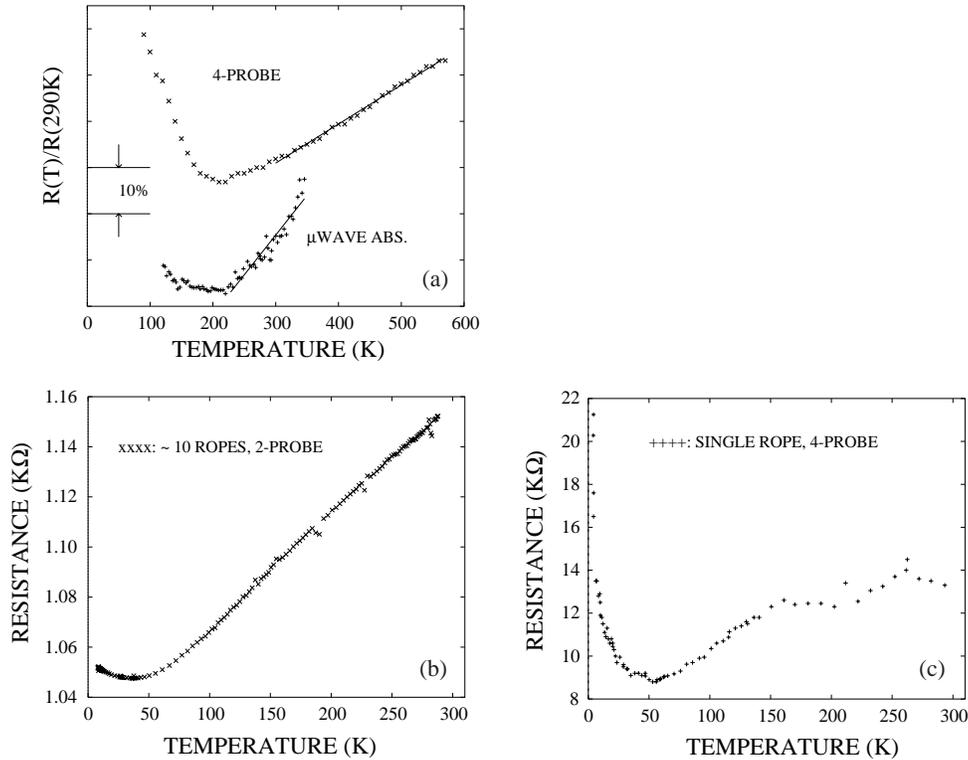
Fig. 2. – Measured resistivities of samples of carbon nanotubes. (a) Bulk material: The top curve is a 4-probe measurement. The lower curve is measured by microwave absorption. (b) 2-probe measurement on several ropes in parallel. (c) 4-terminal measurement of a single rope.
