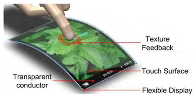
Fig. 95 Graphene-based electrostatic tactile display. Adapted from ref. 1758.
